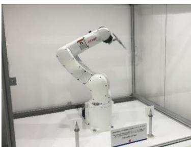
VS-060 is a 6-axis vertical multi-articulated industrial robot that achieves the class top level high-speed performance with a 4kg capacity. From a standard assembly and transport to a surface inspection of the product of complexed shape (curved, etc.), or to works such as polishing and screws tightening, all of these can be done with its advanced technology that is comparable to the work of skilled workers.
