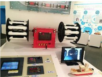
"Full-Automatic Squid-Fishing Machine" is a revolutionary product that has successfully automated the whole process of squid fishing by using the computer, developed at a time when successors of squid fishing have become scarce.
