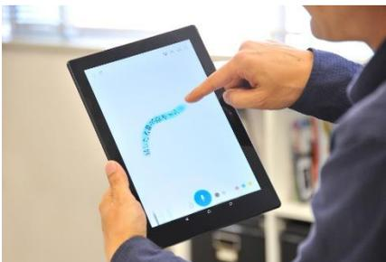
"User Interface for Voice-activated Drawing" is a voice recognition displaying technology that allows spoken words to be displayed on a screen where touched by a fingertip.
