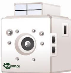
“eyeSWITCH” is a switch that uses the movements of your eyes (eyeballs and eyelids). With the use of call devices, environment control devices, and communication devices, we can call, operate household appliances, and communicate. The device is small, does not need to be attached to the body, and can also be used in the dark.
