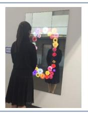
This is a digital signage system that cultivates new dimension for space effecting and image expression by merging mirrors, TV and touch sensor. It is possible to do touch operations through existing glasses.
