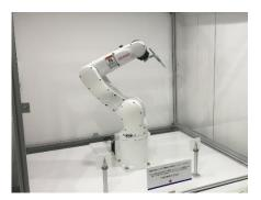
"VS-060" is a 6-axis vertical multi-articulated industrial robot, that achieves the class top level high-speed performance with a load capacity of 4kg.
